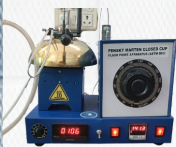
Pensky Marten Closed cup lash point appartus ASTM D93
